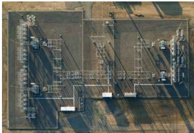
Solar Blue | Stratford, California | 34.5/230kV, 250MVA
