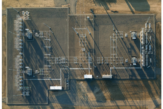
Solar Blue | Stratford, California | 34.5/230kV, 250MVA
