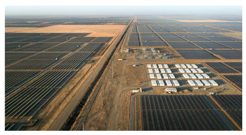
**Solar Blue** | 250MW | 900MWh | 34.5/230kV, 250MVA
