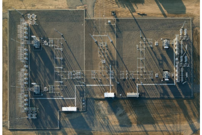
Solar Blue | Stratford, California | 34.5/230kV, 250MVA
